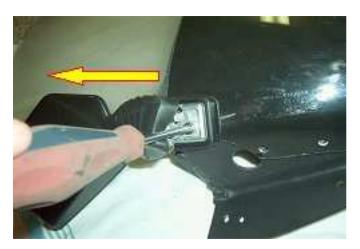
**Step 8** - Push the mirror rearward so it pivots out of the way **just enough** to gain access to the front screw hole. Insert the second screw and align it to the hole in the windshield. Place the screwdriver into the head of the screws. The screwdriver can be allowed to compress into the front of the boot, as shown. Fasten the screw down completely. Pivot the mirror forward again to access the rear bolt. Tighten the rear bolt down completely.
