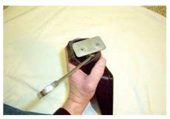
**Step 6 - WITHOUT PULLING ON THE SIDE OF THE BOOT**, slide the wrench into the boot and onto the head of the nut as shown. While holding the metal mounting plate **only**, tighten the nut until it is snug, but still allows the bottom mounting plate to pivot somewhat freely.
