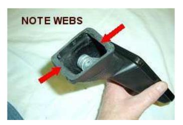
**Step 5** - Make sure the post is centrally located inside the new boot. This may require putting the new boot on, checking location, take boot off, then move post and re-install boot. Install the reproduction boot in the same position that the old one was removed. Make sure the boot is positioned properly as shown above. Please note the webs. These webs are referenced further in the instructions.
