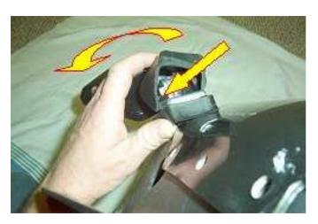
**Step 9 -** Pivot the mirror back **slightly** more as shown above to allow the wrench to access the arm pivot bolt. **DO NOT PIVOT ALL THE WAY BACK.** While keeping the mirror pushed slightly back as shown in the picture above, obtain the Boxed or Open End wrench and place into the opening indicated by the straight arrow. Tighten the post bolt until it is snug enough to allow normal mirror adjustment.
