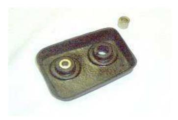
**Step 4 -** Remove the metal spacers from the OEM base pads and install them in the reproduction base pads as shown above.
